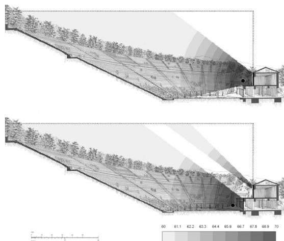
*Fig. 5: Source on the proskenion in Epidaurus (above), then on the orchestra (below), where we see that the reflection off the skene does not reach the audience; transparent program map of a cross-section of the theatre in Epidaurus (diagram hereafter [5]).*
