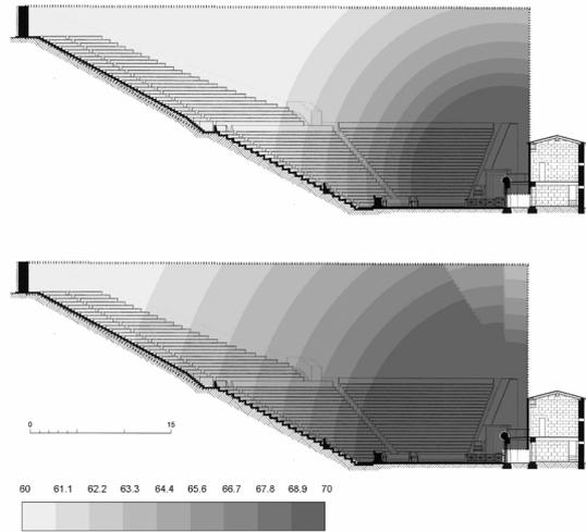
Fig. 2: Only direct sound (above), then added to the reflections off the orchestra and off the skene (below); transparent program map of a cross-section of the theatre in Priene (diagram hereafter [8]).
