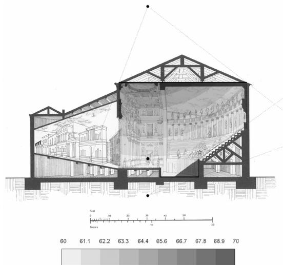
*Fig. 6: Reflections off the roof and the orchestra pit in Palladio's theatre. From this position of the source, 2 metres away from the edge of the stage, the reflection off the orchestra does not even reach the first few rows, while the delay time of the reflection off the ceiling is exactly 50 milliseconds; transparent program map of a cross-section of the Olympic Theatre (diagram hereafter [6]).*
