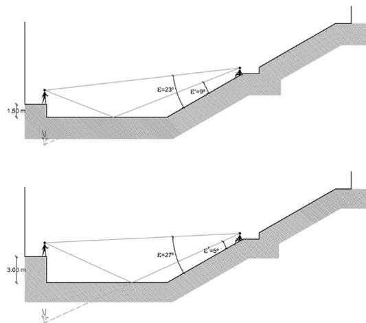
*Fig. 4: If we raise the proskenion, the angle  $\epsilon$  of incidence of the direct sound to the audience increases, but the angle  $\epsilon'$  of incidence of the reflected sound decreases.*
