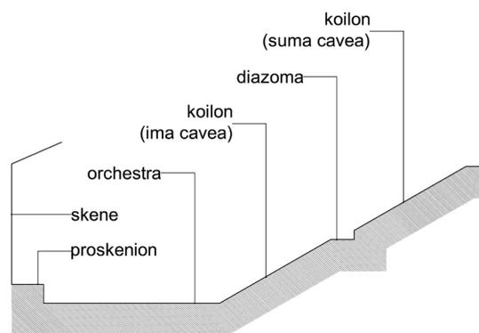
Fig. 1: Longitudinal cross-section of the theatre, with a *diazoma* dividing the tiers.
