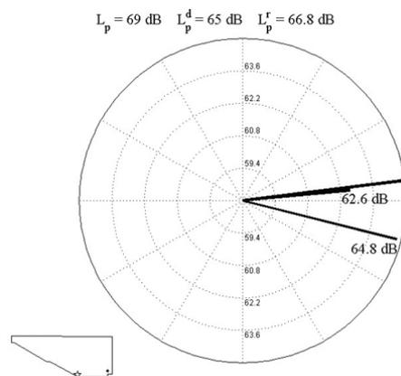
*Fig. 3: Polar diagram from the program, for someone sitting in the first row of the theatre in Priene, with a source on the edge of the proskenion; the reflections off the skene (62.6 dB) and off the orchestra (64.8 dB) give a higher level of reflection (66.8 dB) than the level of direct sound (65 dB).*
