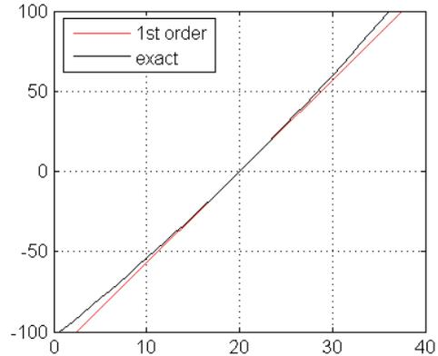
Figure 2: Transmitted power in  $\text{Wm}^{-2}$  according to Stefan-Boltzmann law and its 1<sup>st</sup> order approximation computed in the region of 20°C, (293.15 K)
