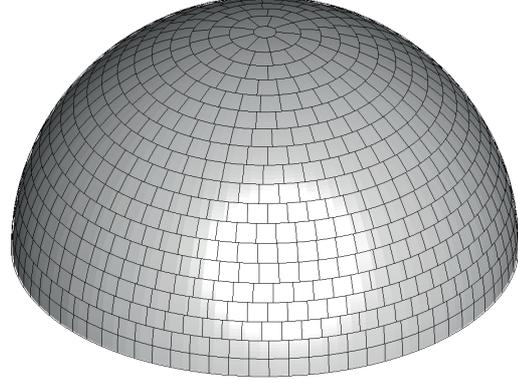
Figure 1: Hemispherical dome containing 1000 equal area cells
