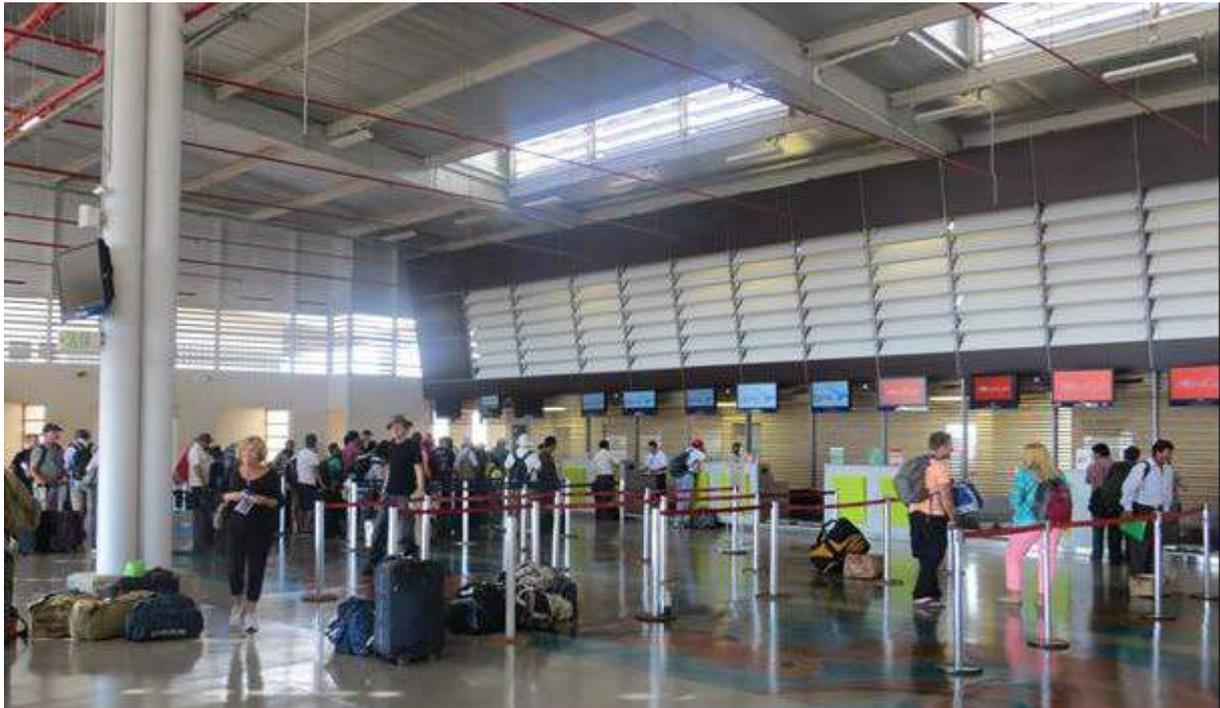
Figure 13. Check-in area, showing good daylight distribution and louvers above the check-in stands to direct natural airflow over the queuing passengers.
