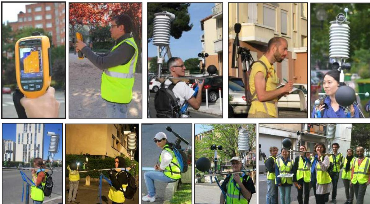
Figure 3 : EUREQUA Project, in-situ experiment; urban climate, air quality and acoustic mobile sensors
