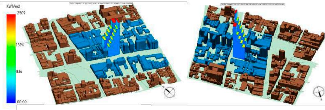
Figure 26: BD Bacatá sunlight and irradiation hours during the whole year
