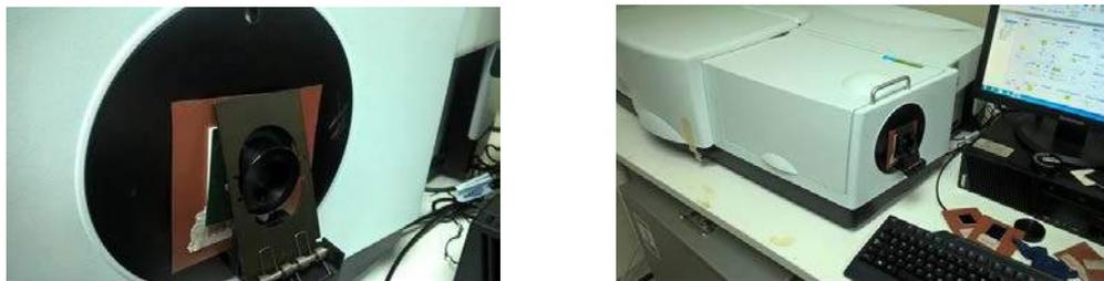
Figure 12: spectrophotometer UV/Vis/NIR PerkinElmer used in the analysis
