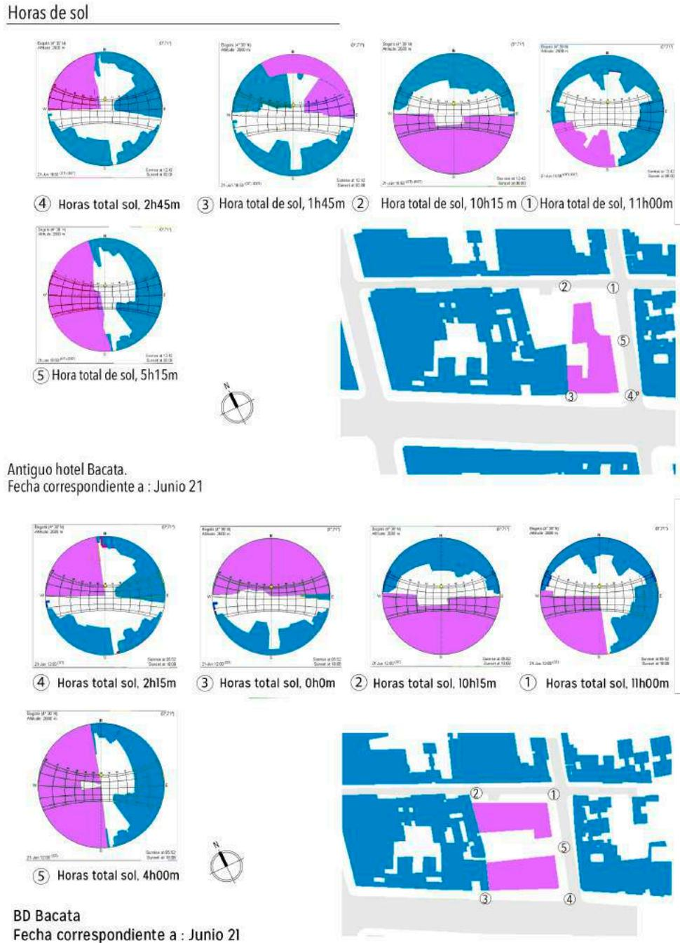
Figure 20: Comparison of sun hours on sidewalks on June 21st
