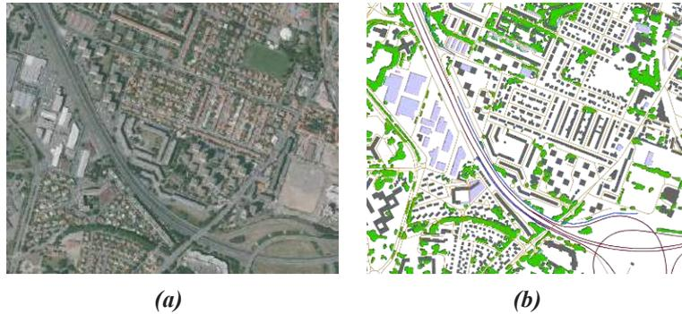
Figure 1 : EUREQUA Project, district of Bordelongue in the city of Toulouse (F); (a) satellite view ([www.geoportail.gouv.fr](http://www.geoportail.gouv.fr)) ; (b) cartographic representation after importation from IGN database via OrbisGIS, SIG validation and vegetation enrichment (<http://orbisgis.org>)
