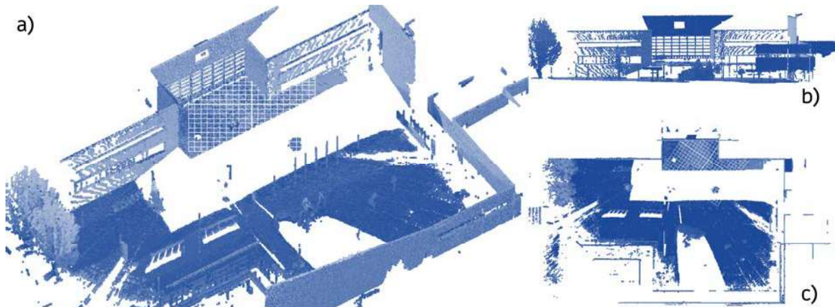
Fig. 5. Geometric reconstruction from LiDAR survey in ReCap Pro: (a) 3D isometric view; (b) orthographic front view; and (c) top view (authors' elaboration).
